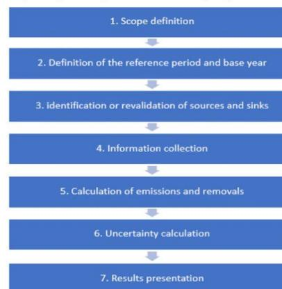
Fig. 1: Steps for the survey of GHG emissions
